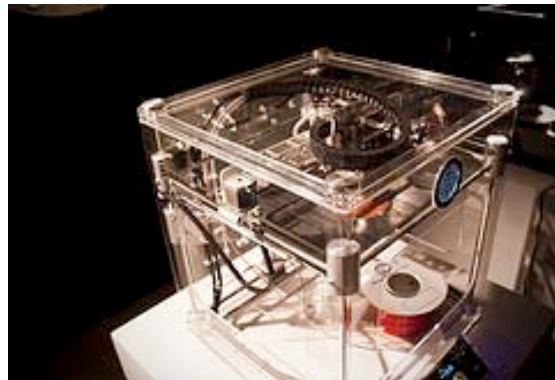
#4: the transparent structure of this 3D printer allows for a detailed look at the printing process
