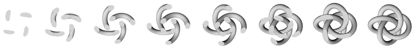
Figure 2: All FOC textiles are produced by literally stacking tiny layers of Polyamide powder in order to form solid objects. Here you can see one link of the Mobius pattern and how the layers are stacked on each other by a Laser Sintering process.
