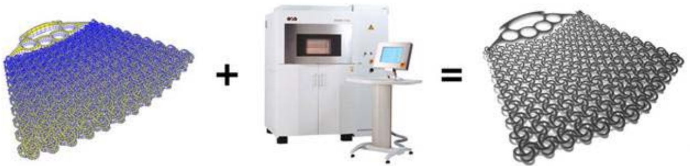
Figure 3: This image shows the steps needed to produce a ready product: 3D CAD file + Laser Sintering machine = ready product
